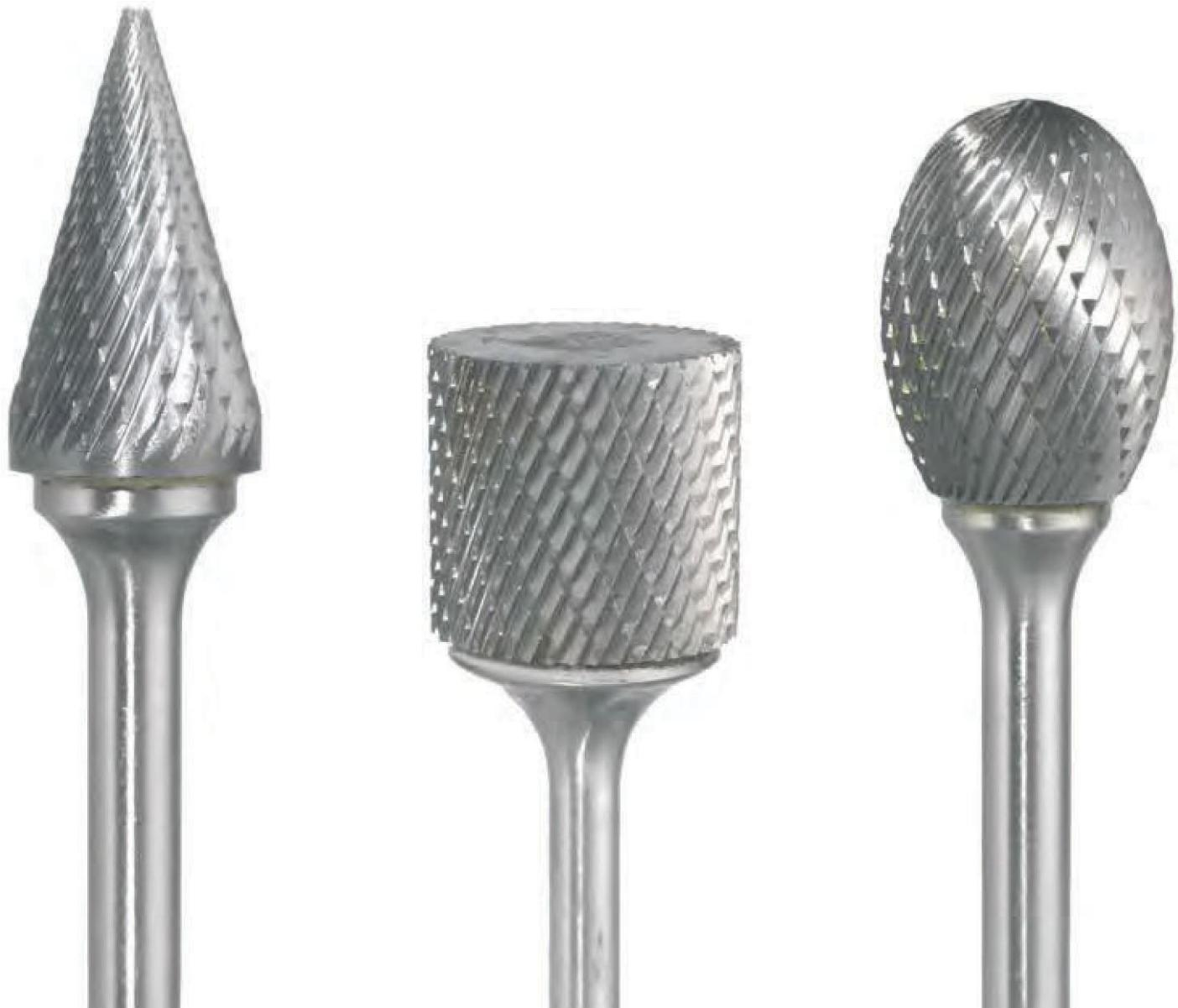
Rotary burrs with chip breaker and standard cutting edge are used in fast machining welds, burrs, plane smoothing, chamfering and other similar operations related with metal machining.
